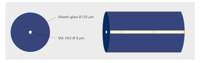
Wavelengths of 1310 nm, 1550 nm or 1625 nm are typically used for transmission with single-mode fibers.
